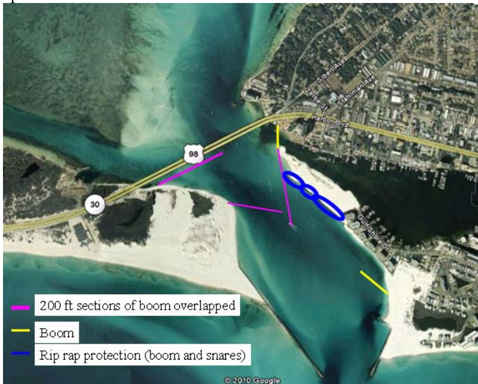
Figure 1. East Pass Boom Configuration
