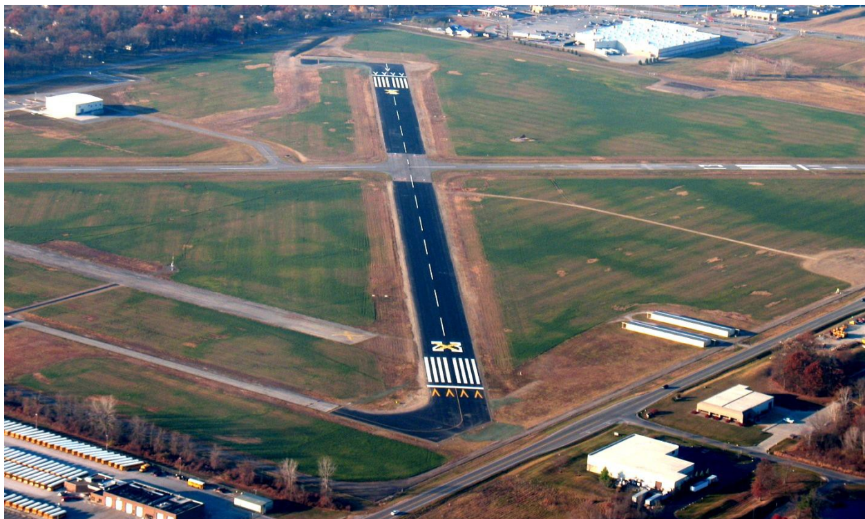
Figure 2-3. Markings for a Temporarily Closed Runway
